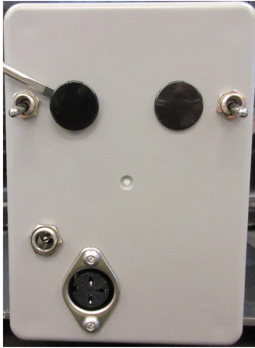
Figure 3.2.1 Removing Access Hole Plugs
