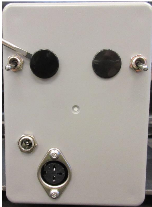
Figure 3.2.1 Removing Access Hole Plugs
