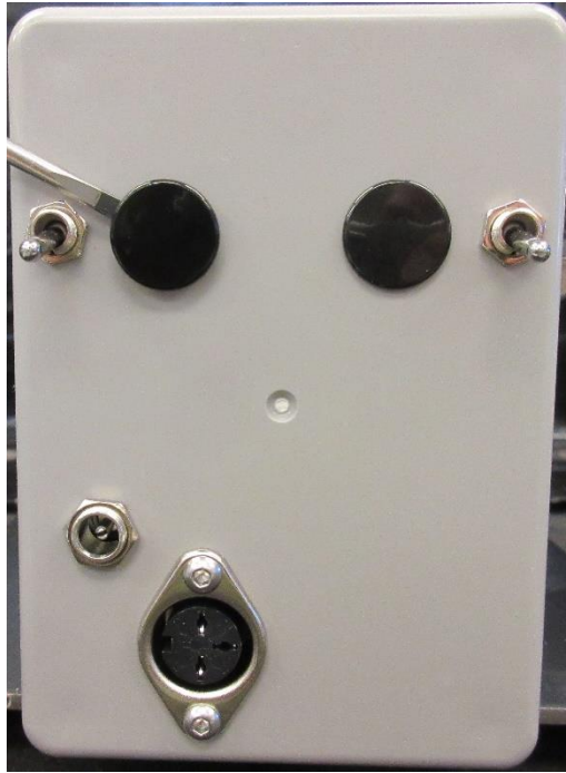
Figure 3.2.1: Removing Access Hole Plugs
