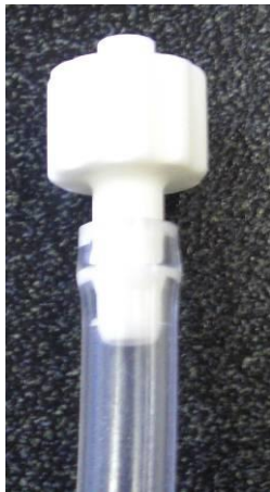
Figure 6 Unadjusted Stop Gate
