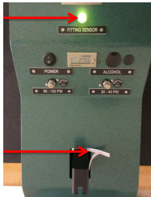
Figure 9.1 – Verifying LFS light "ON"
