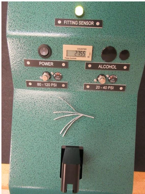
Figure 2.7.3 5 strips of paper for gauge
