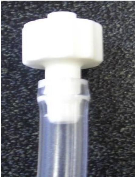
Figure 2.6.1 Unadjusted Stop Gate
