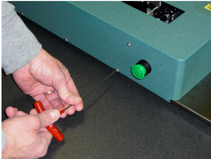
Figure 23: Removing the cover screws
