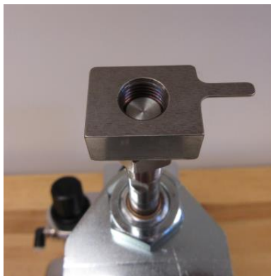
Figure 11: Jaw threaded 1/2-2/3 onto shaft
