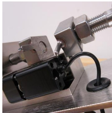
Figure 3.4.13 Jaw threaded on too far And has slipped off jaw block.
