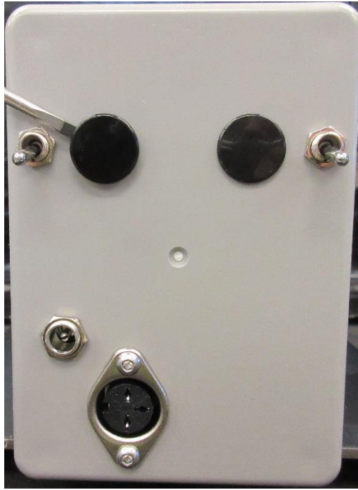
Figure 3.2.1 Removing Access Hole Plugs
