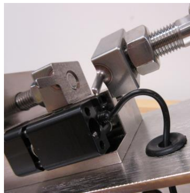
Figure 12: Jaw threaded on too far and has slipped off jaw block
