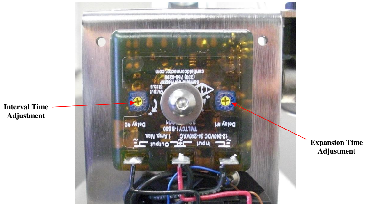
Figure 5: Time Delay Relay and Time Adjustments
